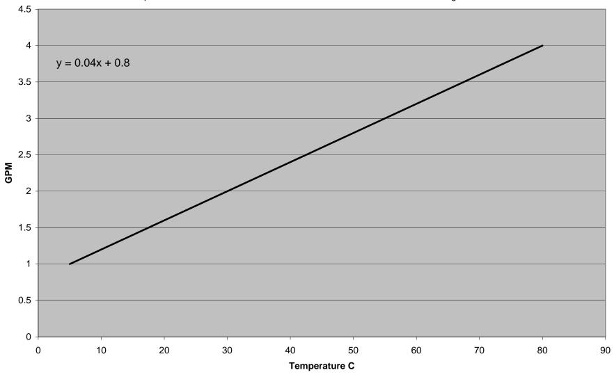
**8730A Series**Coolant pressure into unit should be maintained to achieve correct flow rate but no greater than 100 PSI.
