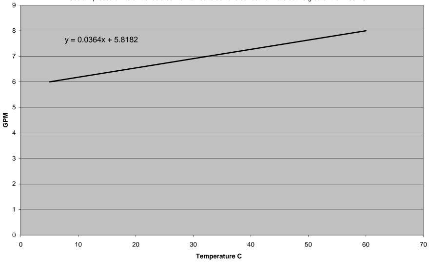
**8755, 8756**Coolant pressure into unit should be maintained to achieve correct flow rate but no greater than 100 PSI.
