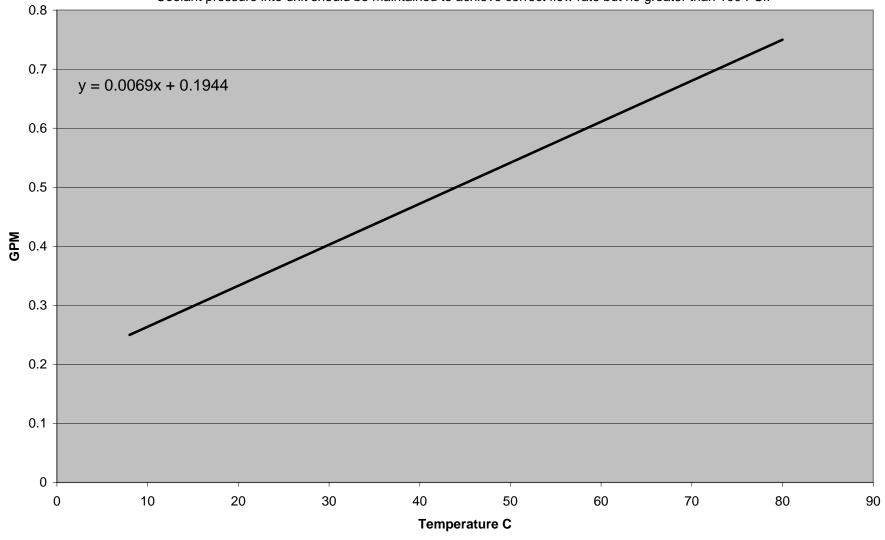
**8720 Series**Coolant pressure into unit should be maintained to achieve correct flow rate but no greater than 100 PSI.
