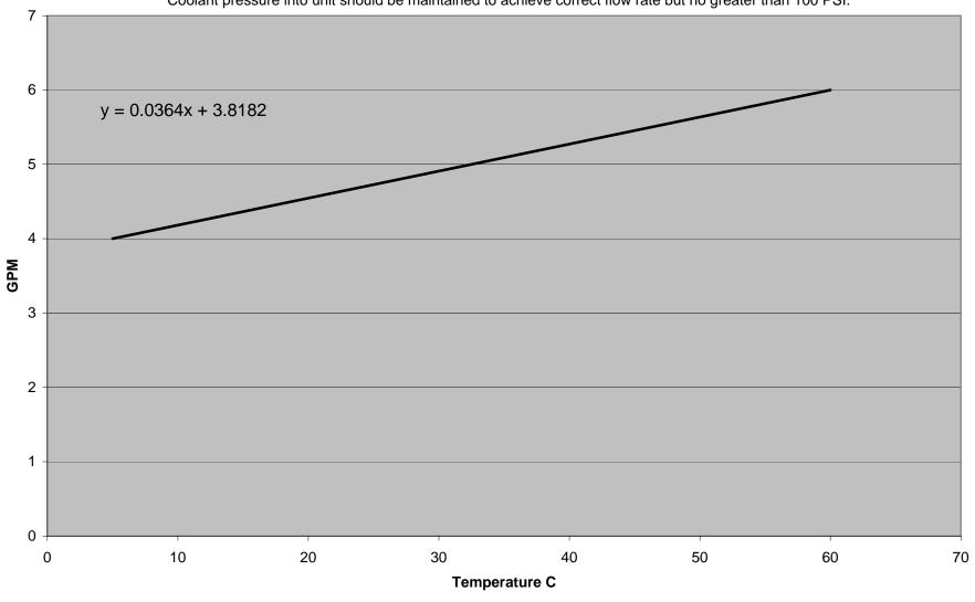
**8745, 8746**Coolant pressure into unit should be maintained to achieve correct flow rate but no greater than 100 PSI.
